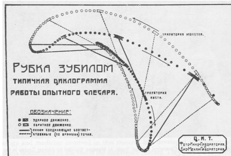
Fig. 1 Top: Strike and pressure: A demonstration of the chronocyclographic method in Gastev's Moscow Institute (C.I.T) by a female worker with an artificial arm. Two photophorescent dots are fixed on the hammer so that the movements can be recorded photographically as curves. On the right side of the picture an assistant holds a measure to provide a scale. Bottom: Diagram of the movements of a worker wielding a hammer. Photos: Reprinted courtesy of Siegfried Zielinski.
